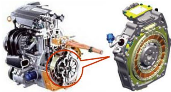
(a) 10-kW motor of the Honda Insight
